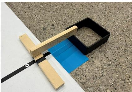
Correct location (One end on each footing, tape mark on footing 1 remains visible)
