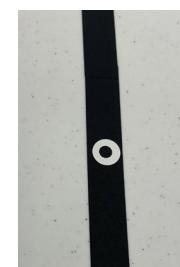
Hole reinforcement stickers are used to mark the test load and footing 1 original locations
